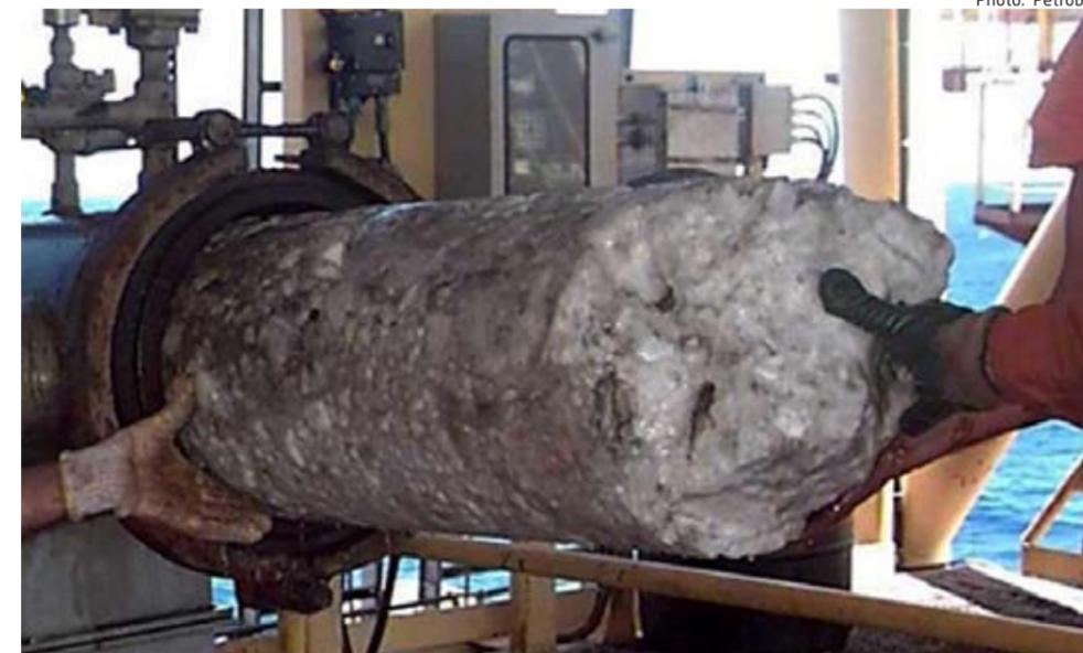
*Gas hydrates are substances resembling snow or ice consisting of water and light hydrocarbons. Under certain conditions they will precipitate in pipes and production gear during oil and gas exploitation. This may again lead to production stops implying major economical losses.*
