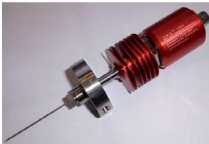
**Figure 3.2** – Picture of an electromagnetic ROLSI™ sampler-injector, showing the actuator and the capillary through which sampling is made.
