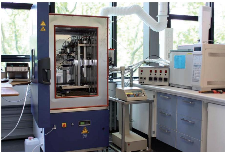
**Figure 4.1** – General aspect of the new developed experimental set-up for the measurement of multi-phase equilibria, showing the cell inside the temperature chamber and the GC unit.
