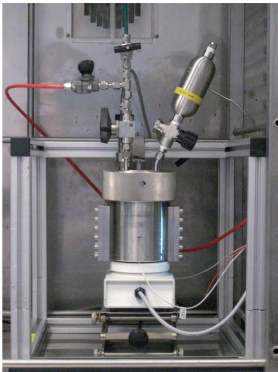
**Figure 5.4** – Image of the high-pressure equilibrium cell together a gas cylinder and other parts, inside the temperature chamber.
