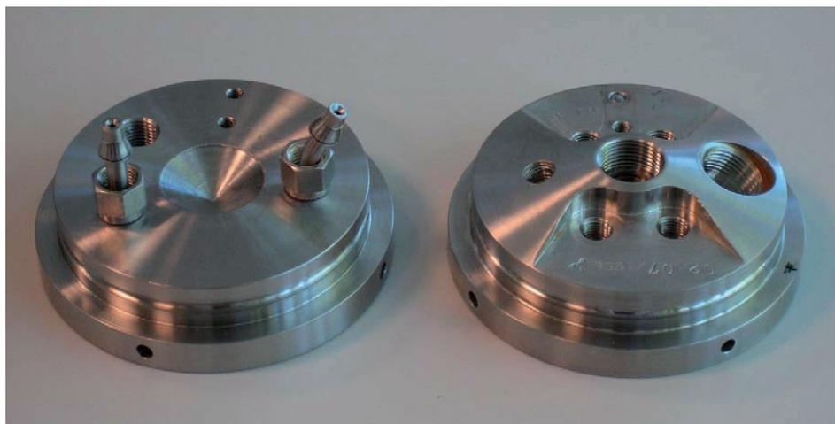
**Figure 5.3** – Lid of the cell. – **On the left:** new lid, with three connections in total, two Swagelok ¼” connections and one connection for the pressure sensor. The two additional small holes visible on top are merely for the support of the cell in its structure. **On the right:** old lid, with seven connections.
