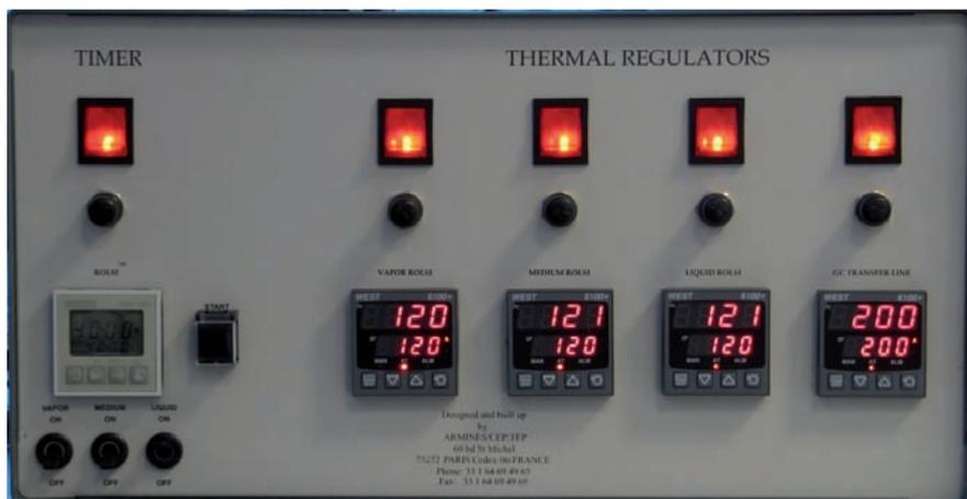
**Figure 4.7** – Control panel for the ROLSI™ samplers, with the timer, the temperature controllers, and additional switches to chose from which valve to use at a given time.
