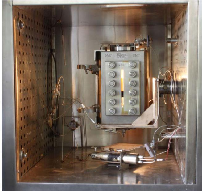
**Figure 4.3: Picture of the DBR JEFRI PVT cell. This is high pressure equipment for phase behavior measurements at various temperatures and pressures. The surrounding steel is the inside of the temperature controlled forced air oven. The cell is monitored on a rocking mechanism suitable for mixing the systems inside the glass chamber. In the middle the glass window is seen which allows visual observations.**
