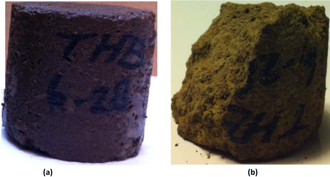
**Figure 7.11 (a) Middle East carbonate reservoir core plug (ME-2) before flooding. (b) Middle East carbonate reservoir core plug (ME-2) after flooding @ 90 °C.**
