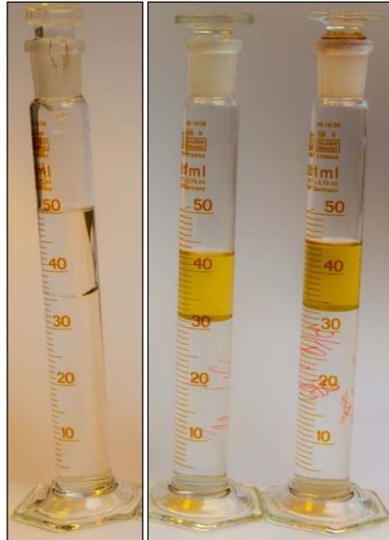
**Figure 5.9 Heptane with different brine solutions after processing in the JEFRI cell at ambient temperature and atmospheric pressure. From left to right heptane with DW (not processed in the JEFRI cell), SW2S and SW3S.**
