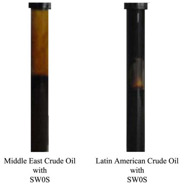
**Figure 5.10** Picture of the formation of a 'gel' phase occurring from hand shaking crude oil and brine solution together. This form is stable as long as the glass tubes are at room temperature and atmospheric pressure. The formed phase is sticky and jelly-like. It is immobile, even though it is not completely solid.
