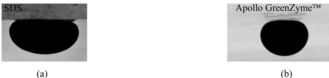
Figure 4: Oil drop shapes under the influence of IFT decreasing components added to the surrounding SW. a – SDS, b – Apollo GreenZyme™.
