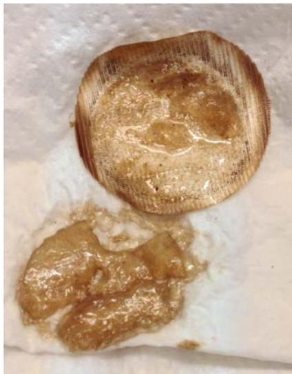
Figure 1: The gel-like formation obtained during crude oil-brine interaction experiments.
