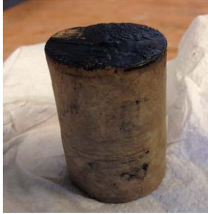
Figure 2: Black precipitation formed at the inlet of the cores in oil displacement experiments when using chalk as core material.
