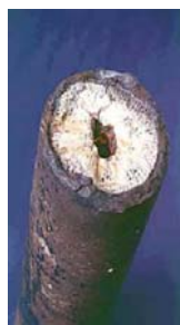
Figure 1-1. Scale formation in a pipe.
