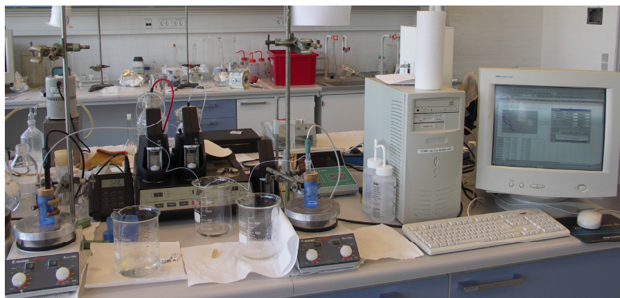
Figure 24: The analysis unit consisting of to titration cells in the left part of the picture and the computer on the right for data acquisition and burette control. The ABU unit is seen behind the titration cells.
