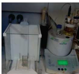
Figure 5.6: Karl Fisher coulometer used for the measurement of water content in hydrocarbon phase.
