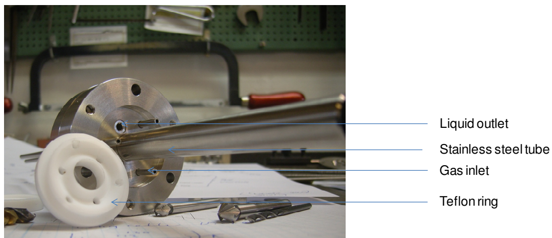
Figure 9-1: Picture of the stainless steel tube, the holding base and the Teflon ring
