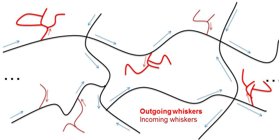
Figure 7.9 Illustrations of the dangling ends and the distance between the whiskers with exiting flow in the infinite cluster. Arrows indicate flux directions, red represents whiskers, and black represents backbones of the infinite cluster.
