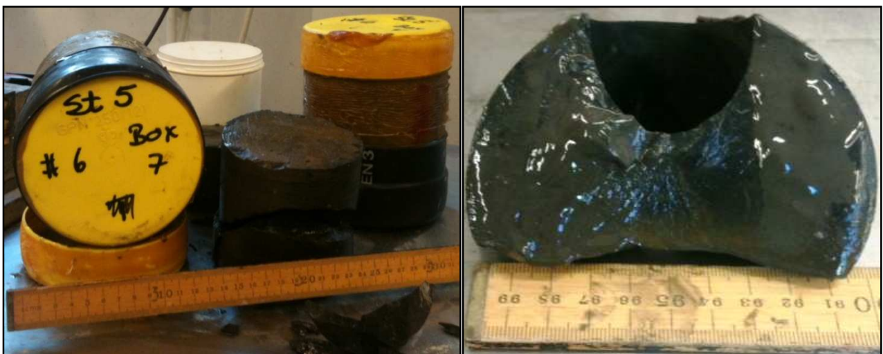
Figure 4.3 Core samples from which plugs were drilled for laboratory testing.
