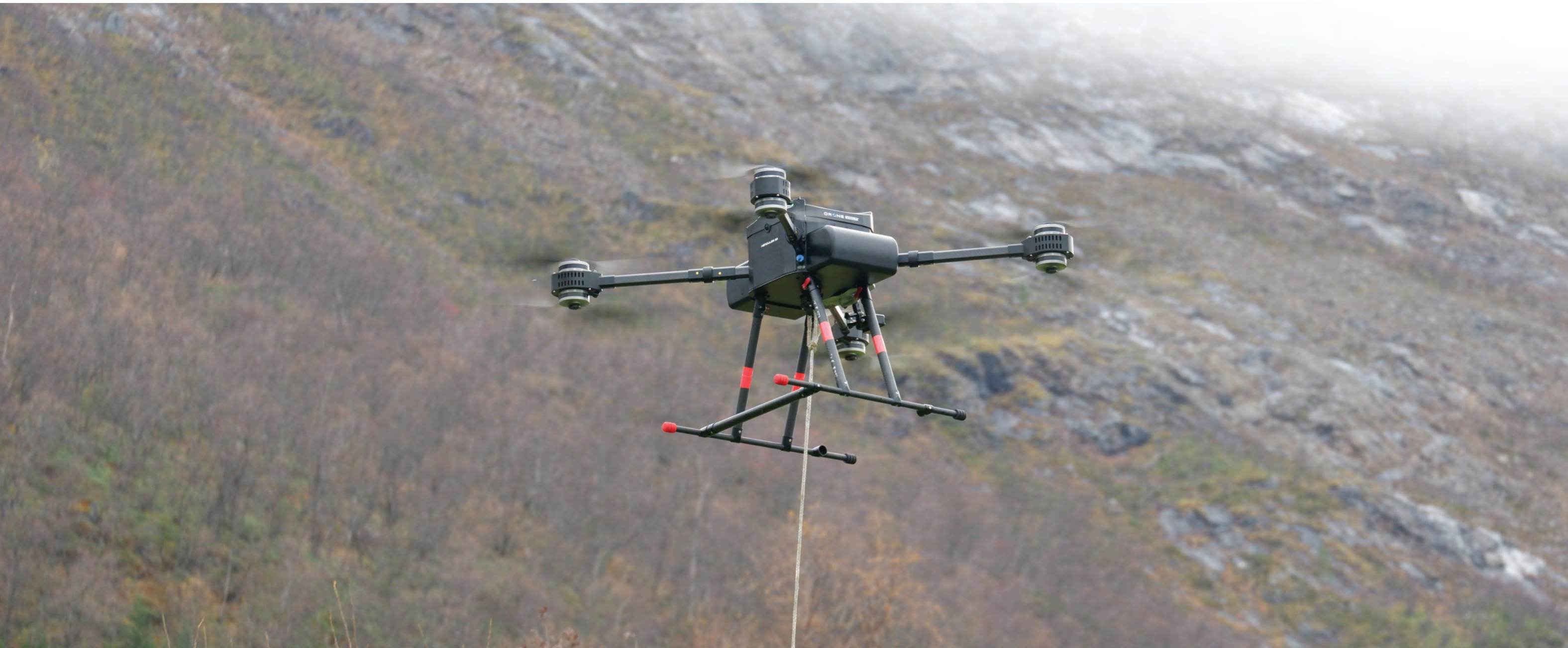
Picture of a heavy-lift drone (Narvik, Norway) used for towing the magnetic payload for mineral exploration purposes.
